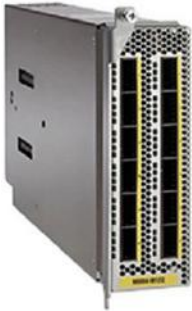
Figure 7. 12-Port 40-Gbps Line-Card Expansion Module
