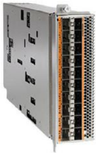
Figure 8. 20-Port 10-Gbps Unified Port Line-Card Expansion Module
