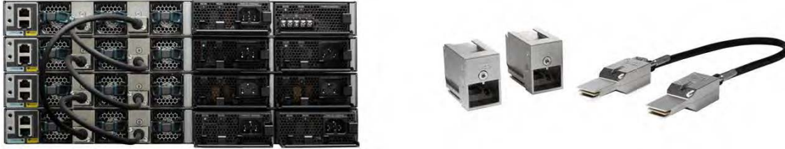
Figure 4. StackWise-160 Kit with Stack Adapters and Cables
