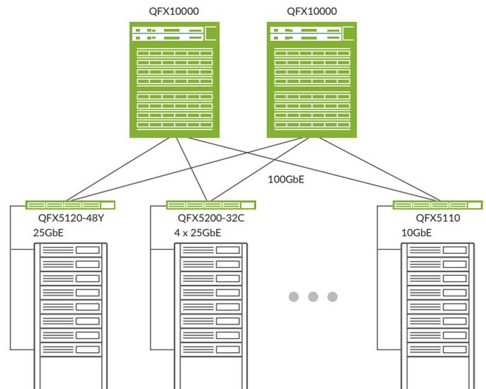
Figure 3. QFX5120-48Y in a leaf-and-spine deployment
