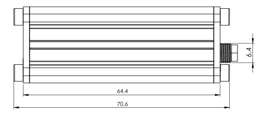
$<sup>*</sup> Housing \ measurements \ are \ presented \ without \ antenna \ connectors \ and \ screws; for \ measurements \ of \ other \ device \ elements \ look \ to \ the \ sections \ below.$
