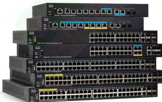
Cisco 350X Series switches are designed to protect your technology investment as your business grows. Unlike switches that claim to be stackable but have elements that are administered and troubleshot separately, the Cisco 350X Series provides true stacking capability, allowing you to configure, manage, and troubleshoot multiple physical switches as a single device and more easily expand your network.
