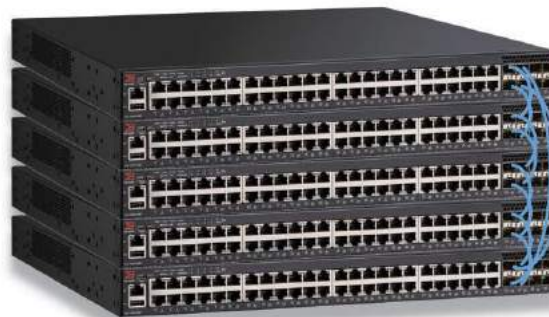
Figure 1: Up to 12 Ruckus ICX 7250 Switches can be stacked together using up to four full-duplex SFP+ 10 Gbps ports for a fully redundant backplane with 480 Gbps of aggregated stacking bandwidth.
