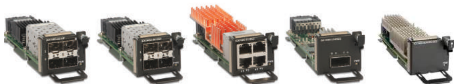
Figure 3: Five different optional port modules are offered for the Ruckus ICX 7450 with a choice of 1 GbE SFP, 10 GbE SFP/SFP+, 10GBASE-T, and 40 GbE QSFP+ options and an IPsec VPN service module.
