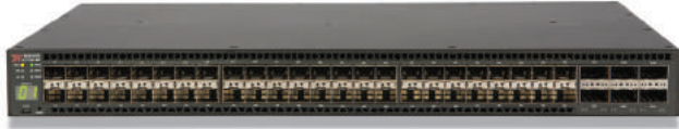
Figure 1: The Ruckus ICX 7750-48F features 48 1/10 GbE SFP+ ports and 6 40 GbE QSFP+ ports that can each be split into 4×10 GbE SFP+ ports. The front panel also displays the unit stacking ID.
