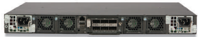
Figure 5: The Ruckus ICX 7750 features hot-swappable redundant power supplies (1+1) and fans (3+1), and an optional 6 40 GbE ports module that can be used for stacking or as additional 40 GbE data ports.
