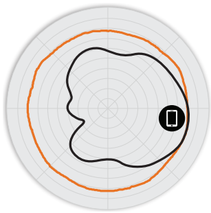
Figure 2. H320 2.4GHz Azimuth Antenna Patterns
