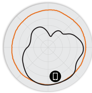
Figure 3. H320 5GHz Azimuth Antenna Patterns
