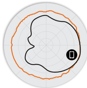
Figure 3. M510 5GHz Azimuth Antenna Patterns
