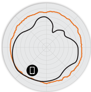
Figure 2. M510 2.4GHz Azimuth Antenna Patterns
