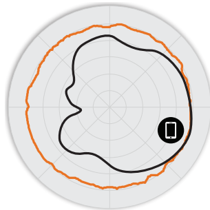
Figure 3. R510 5GHz Azimuth Antenna Patterns
