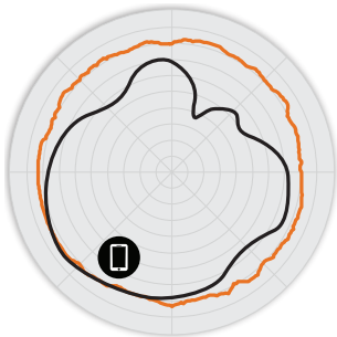
Figure 2. R510 2.4GHz Azimuth Antenna Patterns
