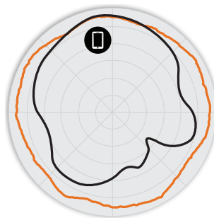
Figure 3. R600 5GHz Azimuth Antenna Patterns
