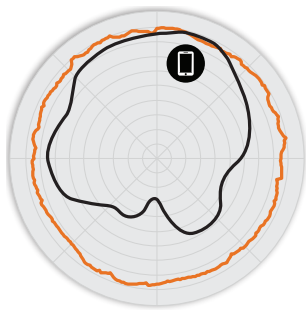
Figure 2. R730 2.4GHz Azimuth Antenna Patterns
