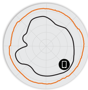
Figure 3. R730 5GHz Azimuth Antenna Patterns
