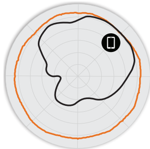
Figure 3. T300 5GHz Azimuth Antenna Patterns
