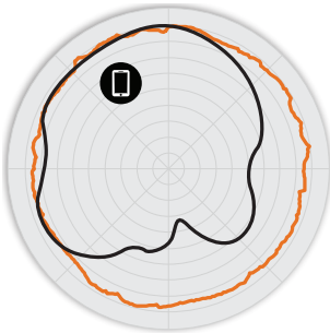
Figure 2. T610o 2.4GHz Azimuth Antenna Patterns
