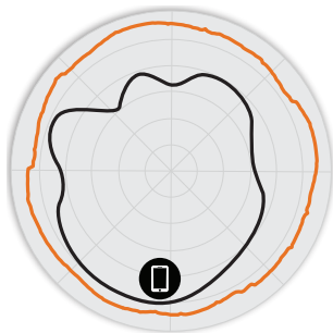
Figure 2. T811 2.4GHz Azimuth Antenna Patterns
