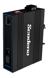
1 Port 10/100Mbps POE+ 1 Port Fiber Uplink, Single mode, Single fiber, SC, 20KM Din rail, Support IEEE802.3af/at, Dual Power DC 48-57V, Each port support Max 30W -40°C to +75°C
