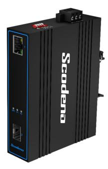
1 Port 10/100Mbps RJ45 + 1 Port SFP slot, Din rail, Dual Power 12-58VDC input, Working Temperature -40°C to +75°C
