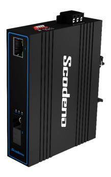
1 Port 10/100Mbps RJ45, 1 Port Fiber Uplink, Single mode, Single fiber, SC, 20KM Din rail, Dual Power 12-58VDC input, Working Temperature -40°C to +75°C
