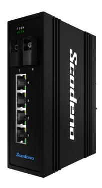
4 Port 10/100Mbps RJ45, 2 SC Port, Single Mode, Single Fiber, 20KM Din rail, Dual Power 12-58VDC input, Working Temperature -40°C to +75°C
