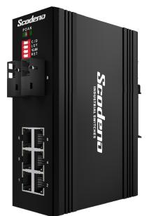
6 Port 10/100Mbps POE, 2 SC Port, Single Mode, Single Fiber, 20KM Din rail, Support IEEE802.3af/at, Dual Power DC48-57V, Each port support Max 30W, -40°C to +75°C
