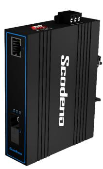
1 Port 10/100/1000 POE+, 1 Port Fiber Uplink, Single mode, Single fiber, SC, 20KM Din rail, Support IEEE802.3af/at, Dual Power DC48-57V, Each port support Max 30W, -40°C to +75°C
