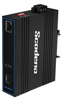
1 Port 10/100/1000 RJ45 + 1 Port Fiber (SFP) Uplink, Din rail, Dual Power 12-58VDC input, Working Temperature -40°C to +75°C
