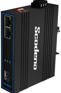
2 Port 10/100/1000 RJ45 + 1 Port Fiber (SFP) Uplink, Dual Power 12-58VDC, Working Temperature -40°C to +75°C
