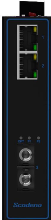
**2 Port 10/100/1000 RJ45, 1 SC Uplink, Single Mode, Dual fiber, 20KM, Din rail, Dual Power 12-58VDC input, Working Temperature -40°C to +75°C**
