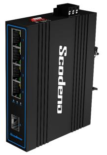
4 Port 10/100/1000 POE+, 1 Port Gigabit Fiber (SFP) Uplink, Din rail, Support IEEE802.3af/at, Dual Power DC48-57V, Each port support Max 30W, -40°C to +75°C
