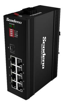
8 Port 10/100/1000 POE+, 1 Port Gigabit Fiber (SFP) Uplink, Din rail, Support IEEE802.3af/at, Dual Power DC48-57V, Each port support Max 30W, -40°C to +75°C
