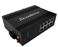
8-ports Gigabit POE Din rail, Support IEEE802.3af/at, Dual Power DC48-57V, Each port support Max 30W, -40°C to +75°C
