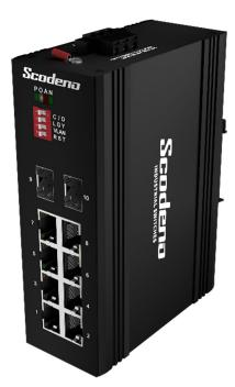
8 Port 10/100/1000 RJ45, 2 Port Gigabit Fiber (SFP) Uplink, Din rail, Dual Power 12-58VDC input, Working Temperature -40°C to +75°C
