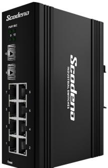
Industrial Layer 2 Switch 8 Port 10/100/1000 PoE, 2x 2.5G SFP Uplink, Din rail, Support IEEE802.3af/at, Ring-Protection Managed, Each port support: Web, CLI, SNMP, VLAN, RSTP/MSTP/ERPS, Dual Power DC48-57V input, Working Temperature -40°C to +75°C
