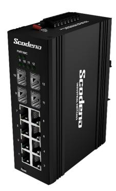
Industrial Layer 2 Switch 8 Port 10/100/1000, 4 Port Gigabit SFP Uplink, Ring-Protection Managed, Web, CLI, SNMP, VLAN, RSTP/MSTP/ERPS, DC12-58V, Working Temperature -40°C to +75°C
