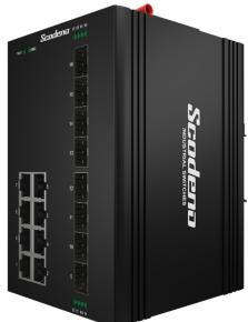
Industrial Layer 2 Switch 8 Port 10/100/1000 +8 Port Gigabit SFP Uplink, Din rail, Ring-Protection Managed, support: Web, CLI, SNMP, VLAN, RSTP/MSTP/ERPS, Dual Power 12-58VDC input, Working Temperature -40°C to +75°C
