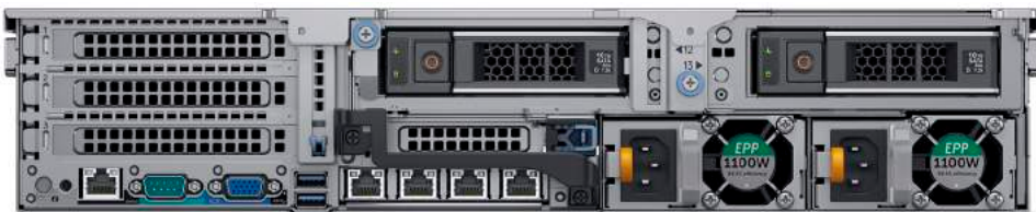
R740xd Rear view - with 4 x 2.5 -inch backplane installed
