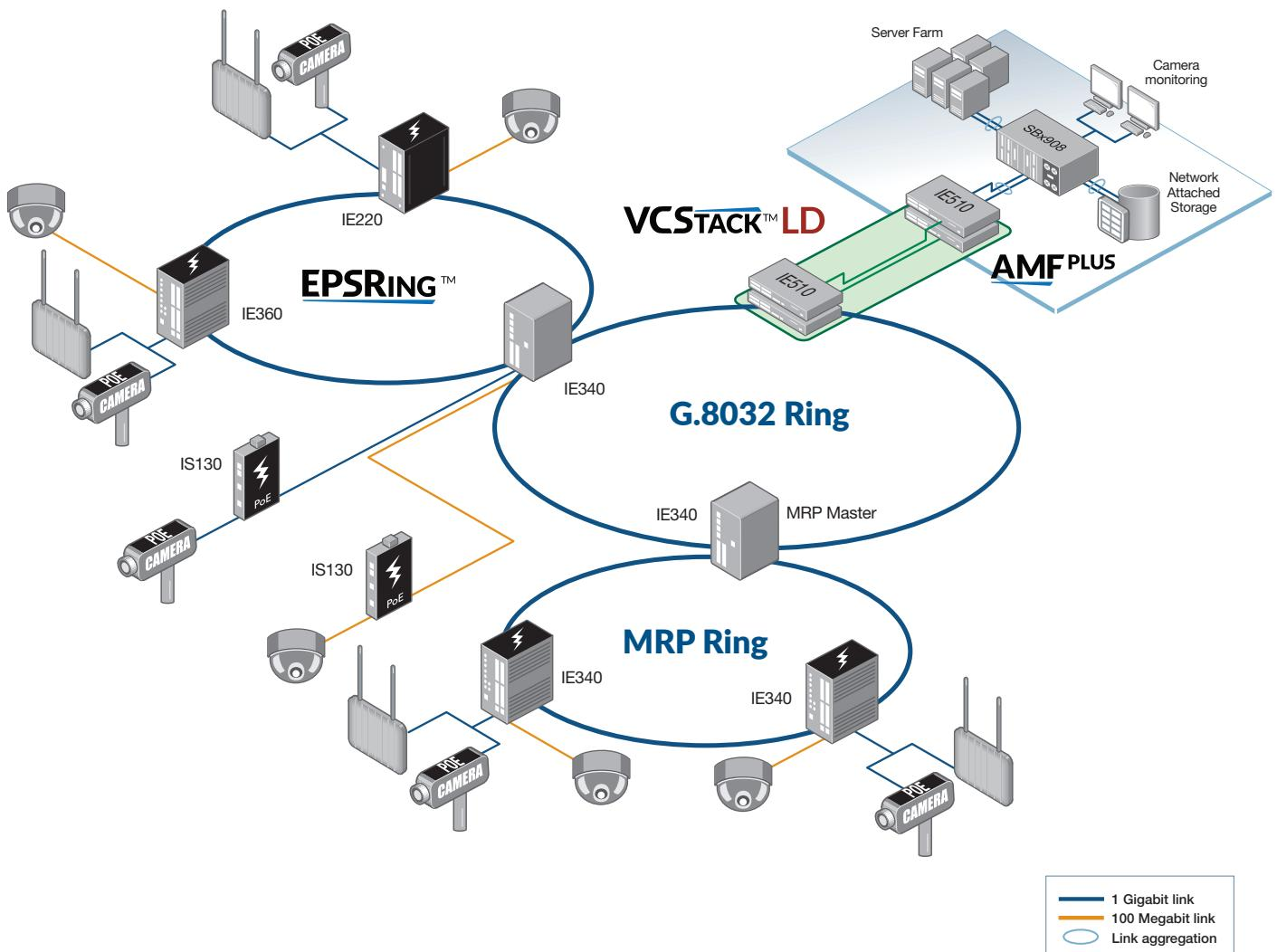
Media Redundancy Protocol (MRP), EPSRing and ERPS (ITU G.8032) provide high-speed resilient ring connectivity. This diagram shows how the IE Series can support a variety of ring network topologies.
