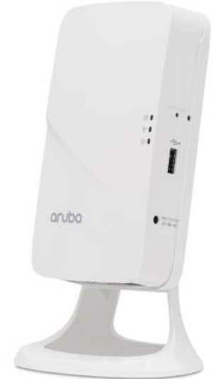
Desk mount (primary remote/branch deployment, using optional desk mount accessory)
