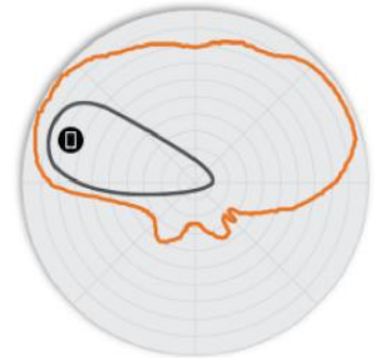
Figure 5. T750 5GHz Elevation Antenna Patterns
