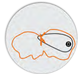
Figure 7. R760 6GHz Elevation Antenna Patterns
