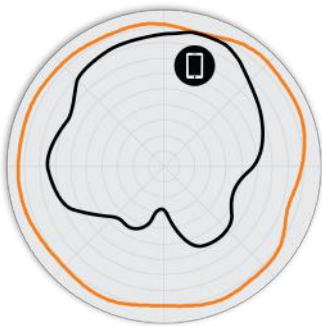
Figure 2. R650 2.4GHz Azimuth Antenna Patterns
