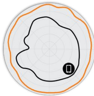
Figure 3. R650 5GHz Azimuth Antenna Patterns
