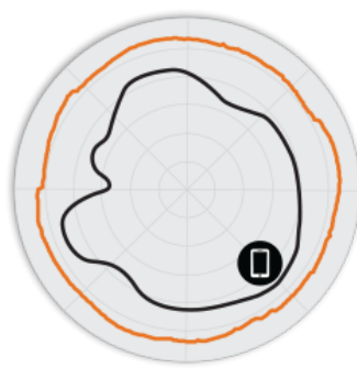
Figure 3. R850 5GHz Azimuth Antenna Patterns
