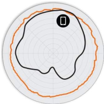
Figure 2. R850 2.4GHz Azimuth Antenna Patterns
