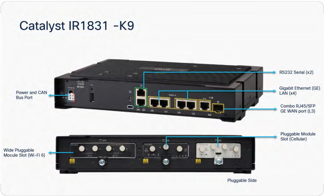
Figure 4. IR1831-K9 interface ports
