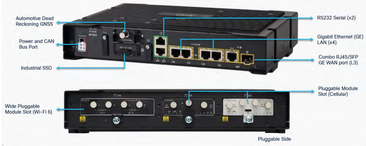
Figure 5. IR1833-K9 interface ports
