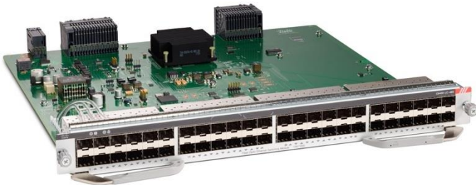
Figure 8. Cisco Catalyst 9400 Series 48-Port 1 Gigabit Ethernet (SFP) Line Card (C9400-LC-48S)
