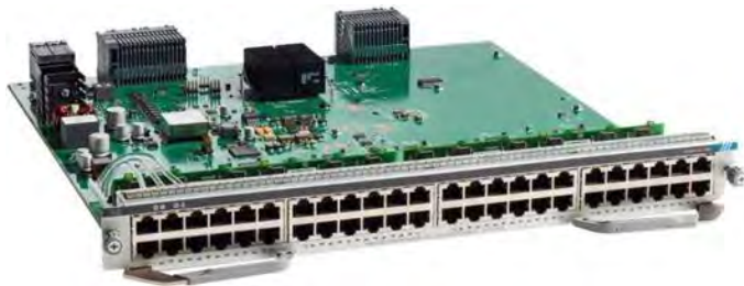
Figure 5. Cisco Catalyst 9400 Series 48-Port UPOE 10/100/1000 (RJ-45) Line Card (C9400-LC-48U)
