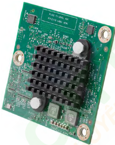
Figure 2. PVDM Enhanced Services Module (SM-X-PVDM)
