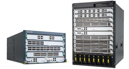
NSS18500 series switches adopts an advanced hardware architecture design. It provides up to 288\*100GE, 272\*40GE, 384\*10GE, 384\*1GE line-rate ports and use an industry-leading Crossbar architecture and provide industrial- grade reliability. The switches support comprehensive data center service features. Their front-to-back airflow design suits data center equipment rooms, and the innovative energy conservation technologies greatly reduce power consumption.
