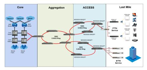
With the rapid growth of triple-play services, higher requirements are put forward for the performance, bandwidth and quality of the ISP Metro Ethernet networks. The NSS5950-32QFP 100G switch have been developed to meet the increasing demand of FTTx services for ISPs. The NSS5950-32QFP provide up to 32-Port 100G interfaces for building backbone network. It will greatly increase the bandwidth and improve the internet experience of end users.
